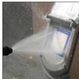
R Series Profile detector sealed to IP69K for extreme wash down conditions
