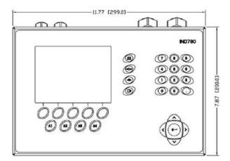
Figure 1-3: Harsh Environment Enclosure Dimensions, Front
