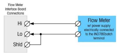
Figure A-80: Non-Isolated Flow Meter Connections
