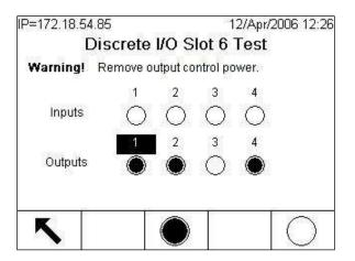
Figure 4-29: Discrete I/O Test Screen
