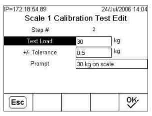
Figure 3-165: Scale 1 Calibration Test Edit Setup Screen
