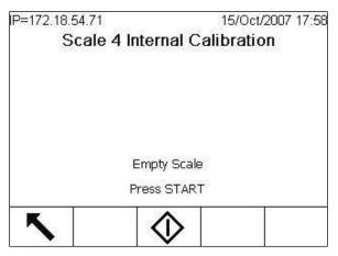
Figure 3-34: Internal Calibration Screen
