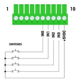
Figure A-85: Example of Active Input from Switches
