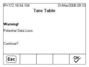
Figure C-9: Tare Table Totalization Data Loss Warning
