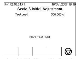
Figure 3-41: Initial Adjustment, Place Test Load
