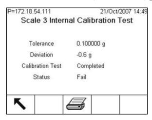
Figure 2-46: Internal Calibration Test Screen, Complete
