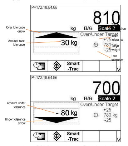
Figure 2-31: Elements of the Over/Under SmartTrac Display
