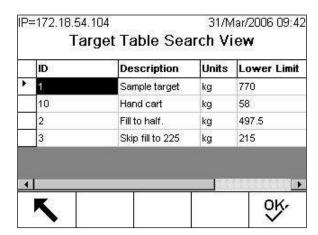
Figure C-26: Target Search View, Over/Under Mode, Weight Value Tolerance Type
