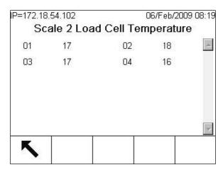
Figure 4-32: Scale Load Cell Temperature Screen
