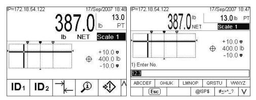
Figure 2-23: Single Scale with SmartTrac and ID Sequence Display
