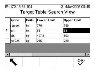
Figure C-27: Target Search View, Over/Under Mode, Weight Value Tolerance Type, Scrolled Right
