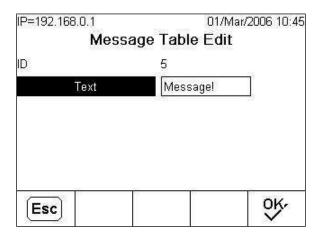
Figure 2-8: Entry Complete—Escape and OK Softkeys Showing
