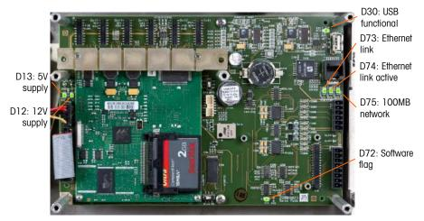
Figure A-39: Main PCB LEDs
