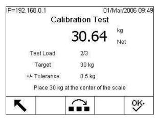
Figure 2-43: Skip Calibration Test Step
