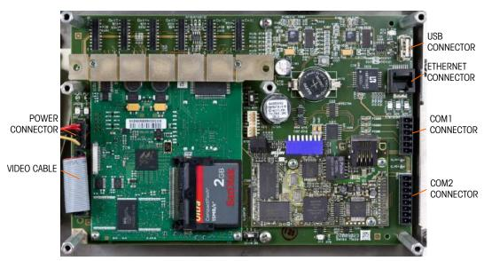
Figure 4-13: Main PCB Connections and Mounting Screws
