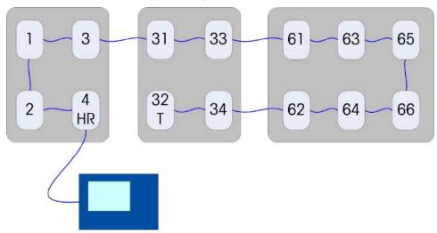
Figure 3-174: Sketch of PDX Cell Network in a Multi-Platform Scale
