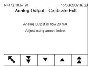
Figure 3-138: Analog Output – Calibrate Full Screen
