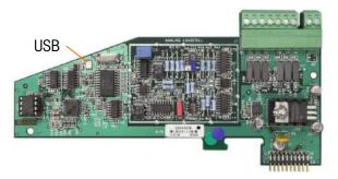
Figure A-45: Analog Load Cell LED
