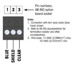
Figure A-97: RIO Connection Wiring
