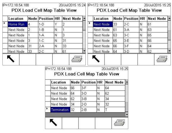
Figure 3-178: Multi-Platform Scale Displayed in Table View
