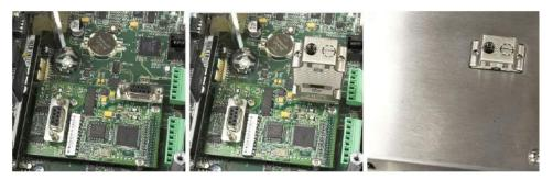
Figure A-110: PROFIBUS PLC Module Connector for Panel Mount Enclosure
