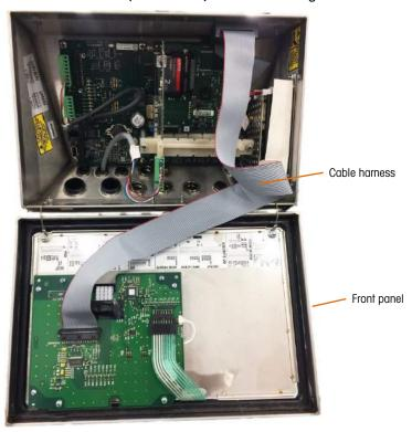
Figure A-11: Front Panel Reversed, Longer Cable Harness Installed
