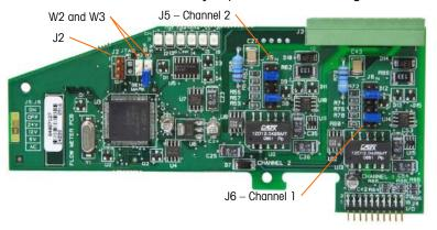
Figure A-78: Flow Meter Interface Board Jumper Locations
