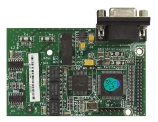
Figure A-107: PROFIBUS PLC Module for Harsh Enclosure
