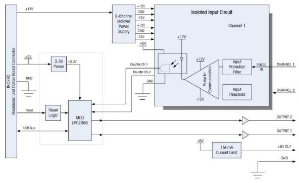
Figure A-77: Block Diagram, Channel 1 Shown
