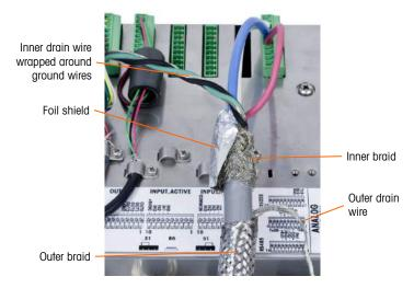
Figure A-67: POWERCELL PDX Home Run Cable, Panel Mount Enclosure
