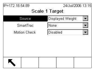
Figure 3-80: Scale Target Screen, Over/Under Mode
