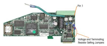
Figure A-46: POWERCELL MTX Option Board
