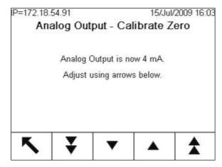
Figure 3-137: Analog Output – Calibrate Zero Screen
