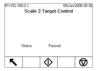
Figure 2-20: Example of Paused State in Target Control
