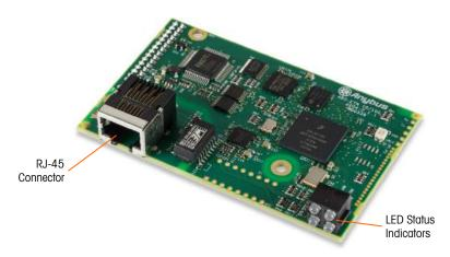
Figure A-111: PROFINET PLC Module Components
