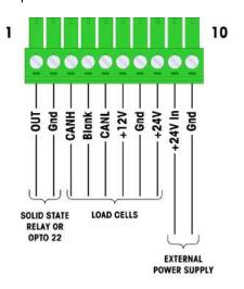
Figure A-52: POWERCELL PDX Option Board Connections
