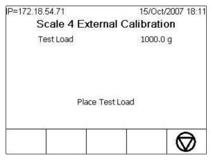
Figure 3-38: External Calibration, Place Test Load
