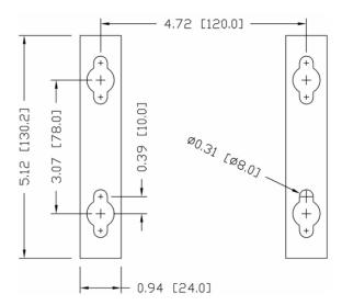
Figure A-14: Mounting Hole Pattern
