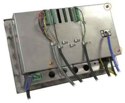
Figure A-1: Opening the Panel Mount Enclosure
