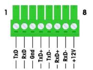
Figure A-35: COM2 Port Connections
