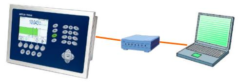
Figure D-2: Connecting the IND780 to a PC with Patch Cables
