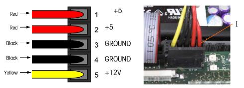
Figure 4-14: Pins on the Power Supply Harness
