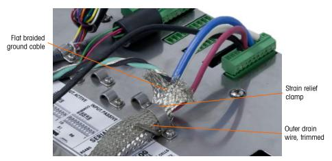
Figure A-68: POWERCELL PDX Home Run Outer Braid Termination, Panel Mount Enclosure
