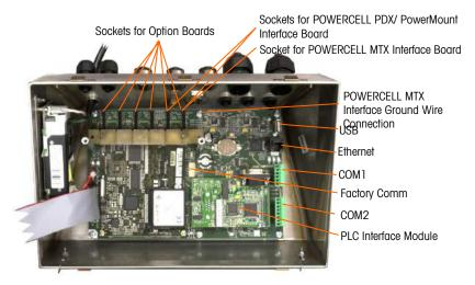
Figure A-29: Wiring Connections, Top View, Harsh Enclosure
