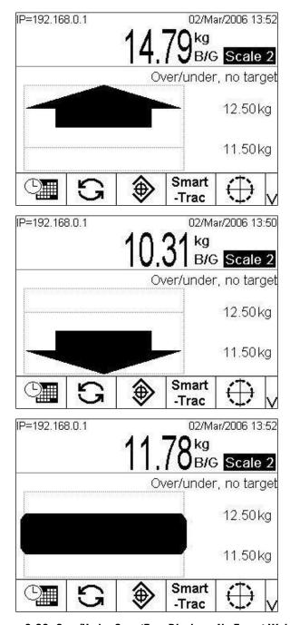
Figure 2-32: Over/Under SmartTrac Displays, No Target Weight
