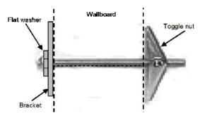
Figure A-17: Wallboard or Drywall Installation
