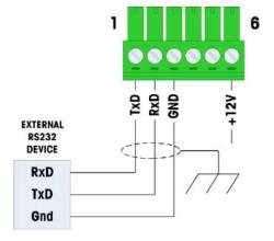
Figure A-34: COM1 Wiring for RS232
