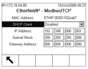
Figure 3-141: EtherNet / IP PLC Interface Setup Screen
