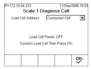
Figure 3-205: Diagnose Cell Connect Cell Screen
