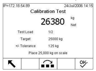
Figure 3-184: Calibration Test Screen
