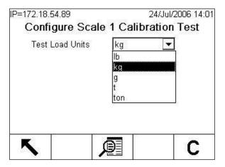
Figure 3-163: Configure Scale 1 Calibration Test Setup Screen
