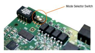
Figure A-84: Discrete I/O Mode Selector Switch, Active Position
