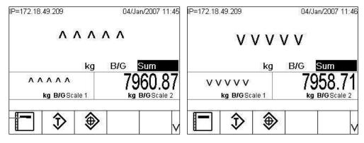
Figure 2-12: Summed Scales Over Capacity (left) and Under Range (right)
