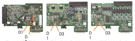
Figure 4-10:3LED Locations: IDNet (left), Serial (center) and DIO (right) Cards
