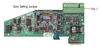
Figure A-41: Analog Load Cell Option Board
