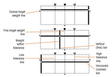
Figure 2-34: Cross Hairs SmartTrac Displays, Off Target
