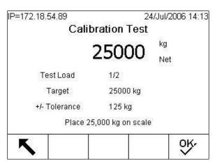
Figure 3-182: Calibration Test Screen
