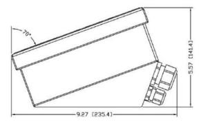
Figure 1-4: Harsh Environment Enclosure Dimensions, Side
