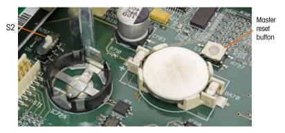
Figure A-38: Main PCB Master Reset Button Location
