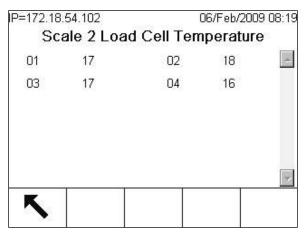
Figure 3-194: Scale Load Cell Temperature Screen
