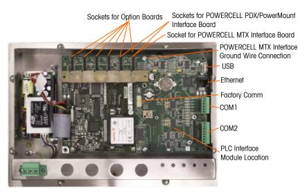
Figure A-30: Wiring Connections, Top View, Panel Mount Enclosure
