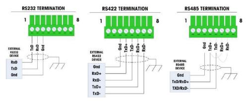
Figure A-36: COM2 Wiring for External Equipment
