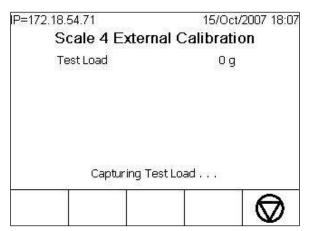
Figure 3-37: External Calibration, Capturing Zero Load
