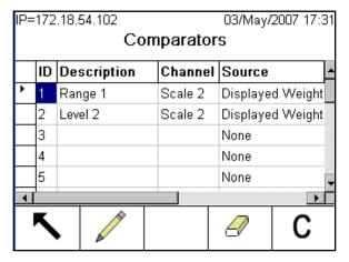
Figure 3-81: Comparator List for Scale 2
