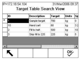
Figure C-22: Target Table Search View, Material Transfer Mode, Target Deviation or % Target Tolerance Type
