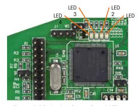
Figure 4-12: Analog Output Board LEDs
