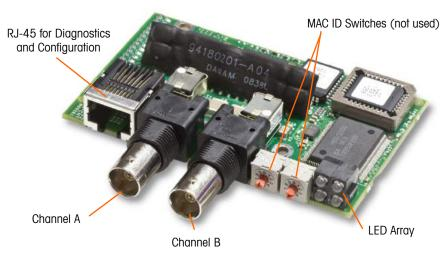
Figure A-99: ControlNet PLC Module Connections and Components
