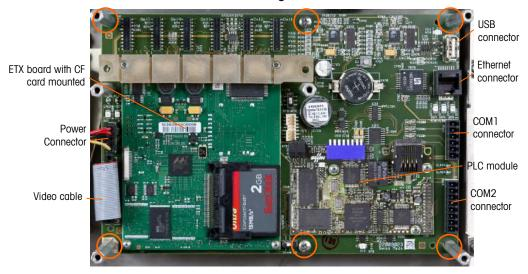
Figure 4-52: Main PCB Connections and Mounting Screws
