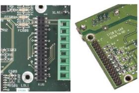
Figure 4-65: PLC Interface Module Socket on Main PCB (left) and Connector Pins on the Underside of a Module (right)
