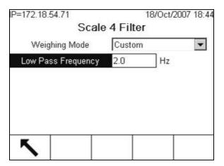
Figure 3-54: Filter Screen Custom Weighing Mode, SICS (WM/WMH)
