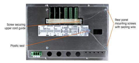
Figure A-119: 3-Point Sealing, Panel Enclosure Rear Cover
