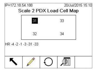
Figure 3-175: Load Cell Map for Scale 2, Configured, Not All Cells Displayed
