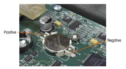
Figure 4-16: Battery Installed
