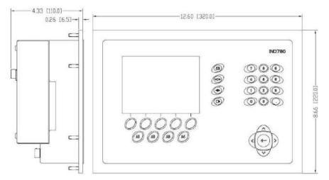
Figure 1-2: IND780 Panel Mount Enclosure Dimensions
