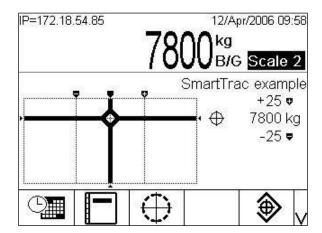
Figure 2-33: Cross Hairs SmartTrac Display, On Target
