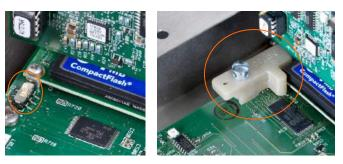
Figure A-113: Metrology Security Switch (left) and Cover Installed (right)
