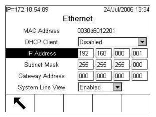
Figure 3-123: Ethernet Setup Screen DHCP Client Disabled
