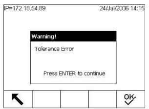
Figure 3-183: Calibration Test Tolerance Error Screen
