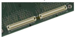
Figure 4-57: Close-Up View of ETX Connectors on Main PCB
