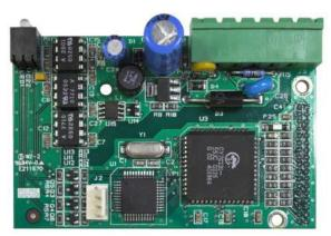
Figure A-102: DeviceNet Option Board
