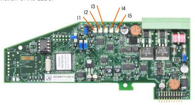
Figure 4-11: Board LEDs
