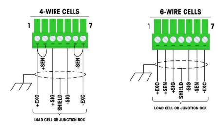
Figure A-43: Load Cell Connections
