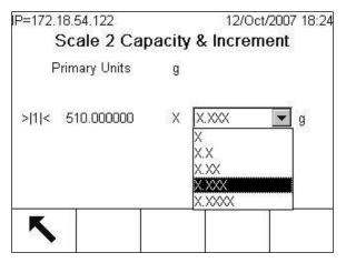
Figure 3-25: Capacity and Increment Setup Screen, SICS
