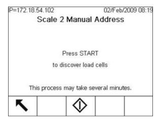
Figure 3-15: Manual Address Start Screen, PDX
