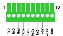
Figure A-92: Serial Option Board Connector
