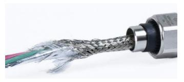
Figure A-59: Inner Sheath Frayed
