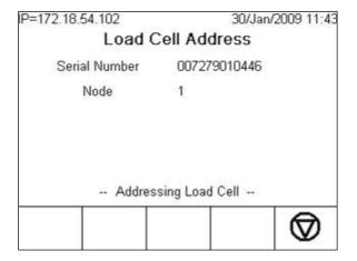
Figure 3-13: Single Cell Addressing Screen, PDX
