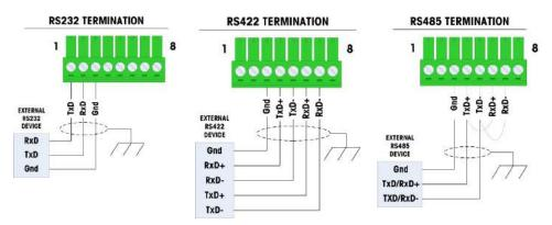
Figure A-93: Connector Terminations for Serial Option Board
