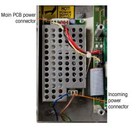
Figure 4-62: Power Supply, Connected
