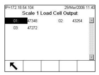
Figure 4-21: Load Cell Output Screen
