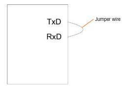
Figure 4-28: Jumper Wire Placed Between the Transmit and Receive Terminals
