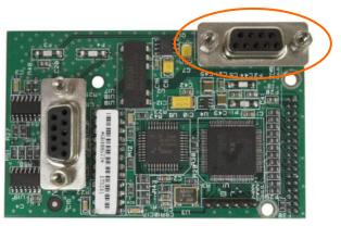
Figure A-109: PROFIBUS PLC Module for Panel Mount Enclosure
