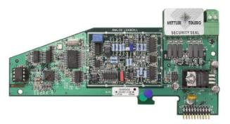
Figure A-115: Security Seal Installed
