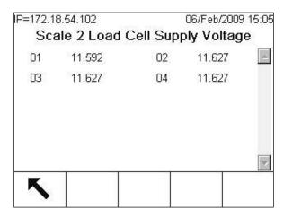
Figure 4-33: Scale Load Cell Supply Voltage Screen
