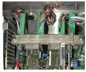
Figure A-23: Shield Wire Termination, Harsh Enclosure
