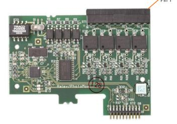
Figure A-82: Discrete I/O Board, Solid State Relay
