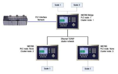
Figure D-14: Example of a Cluster with PLC Interface Sharing
