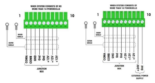
Figure A-48: POWERCELL MTX Option Board Connections
