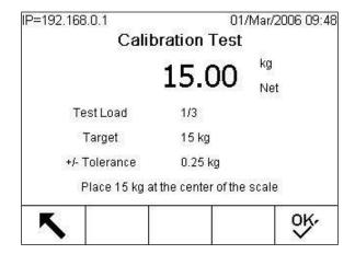
Figure 2-41: Calibration Test Step
