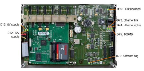
Figure 4-8: Main PCB LEDs
