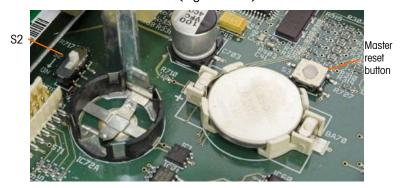
Figure 4-50: Main PCB, Master Reset Button and S2 Locations Indicated
