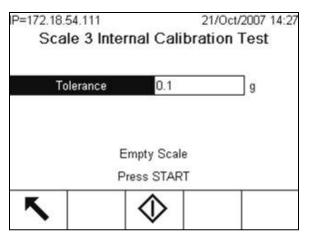
Figure 3-186: Internal Calibration Test Screen
