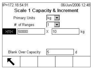
Figure 3-24: Capacity and Increment Setup Screen
