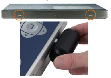
Figure A-2: Opening the Harsh Enclosure, Preferred Method
