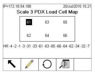
Figure 3-176: Load Cell Map for Scale 3, All Cells Displayed
