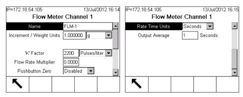
Figure 3-64: Flow Meter Channel Configuration Screen
