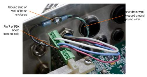
Figure A-66: POWERCELL PDX Home Run Power Ground Connection, Harsh
