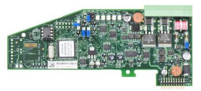
Figure A-51: POWERCELL PDX Option Board
