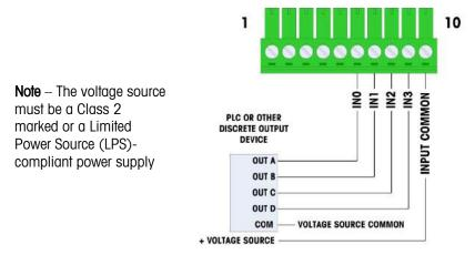
Figure A-86: Example of Passive Input from Discrete Output Device
