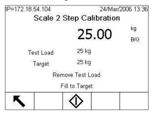
Figure 3-32: Step Calibration, First Step Complete
