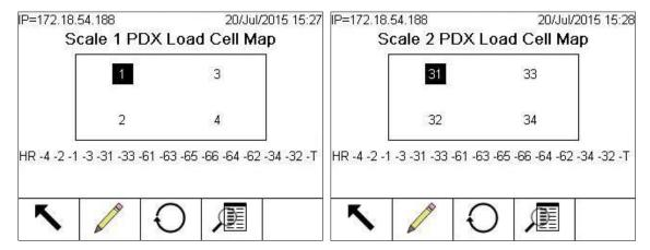
Figure 3-177: Load Cell Maps for Scales 1 and 2, All Cells Displayed
