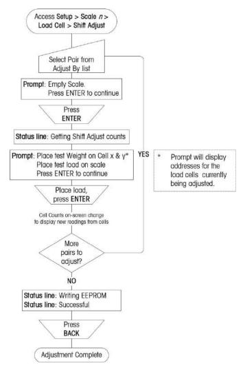
Figure 3-22: Procedure for adjusting cells by pairs
