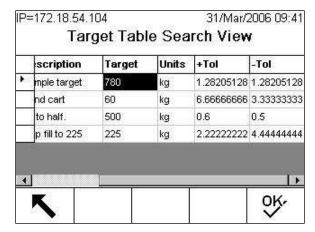
Figure C-25: Target Search View, Over/Under Mode, Target Deviation or % Target Tolerance Type, Scrolled Right
