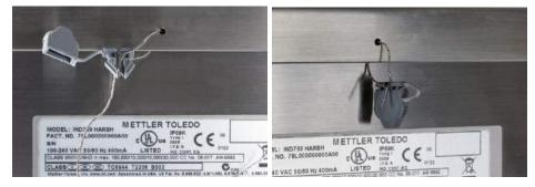
Figure A-122: Final Steps in Sealing Harsh Enclosure
