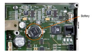
Figure 4-15: Main PCB, Battery Location Indicated
