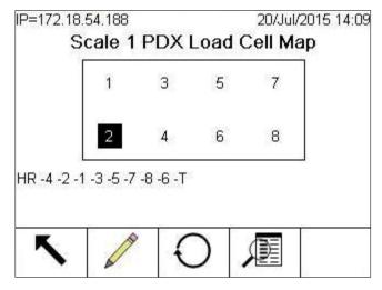
Figure 3-170: Completed PDX Load Cell Map
