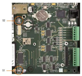
Figure A-37: Main PCB Switch Locations
