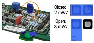
Figure A-42: Analog Load Cell Board Millivolt Jumper Location and Settings
