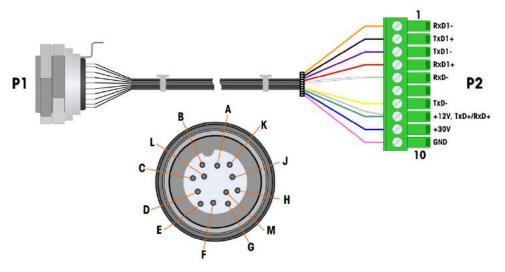
Figure A-90: IDNet Cable for IDNet Option Board
