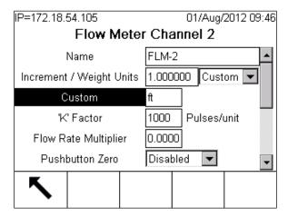
Figure 3-65: Flow Meter Channel Configuration Screen
