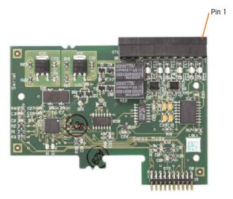
Figure A-91: Serial Option Board
