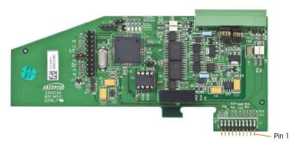
Figure A-94: Dual-Channel Analog Output Option Board
