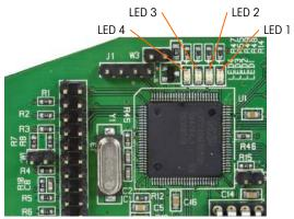
Figure A-96: Analog Output LEDs
