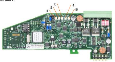
Figure A-74: POWERCELL PDX Board LEDs
