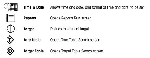
When more than five softkeys are defined, a MORE DOWN symbol **V** displays to the right of the softkeys, as in Figure E-1. Press the DOWN navigation key on the keypad to advance to the second screen of softkeys. (If enough softkeys are defined, a third screen of softkeys is available, and the MORE UP/MORE DOWN symbol (displays in the second screen. Pressing the DOWN navigation key again would scroll to a third screen).
