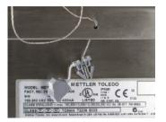
Figure A-121: Sealing Wire Threaded Through Cover and Clip
