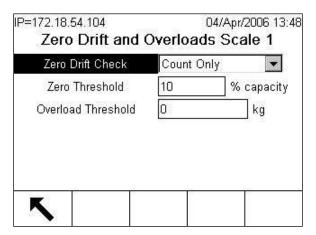
Figure 3-161: Zero Drift and Overloads Screen
