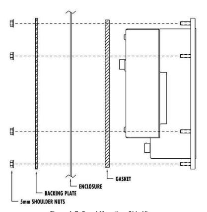
Figure A-7: Panel Mounting, Side View
