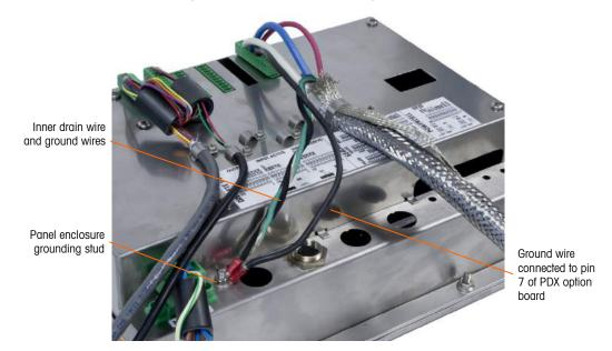
Figure A-69: Completed POWERCELL PDX Home Run Power Ground Connection,
