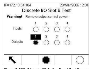
Figure 3-209: Discrete I/O Option Board Test Screen
