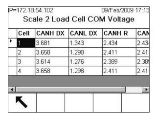
Figure 4-34: Scale Load Cell COM Voltage Screen
