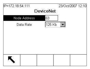
Figure 3-140: DeviceNet PLC Interface Setup Screen
