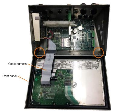
Figure A-9: Harsh Enclosure Open, with Front Panel in Original Orientation
