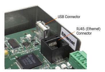
Figure A-32: Ethernet and USB Connections
