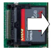
Figure 4-61: CF Card Removal – Original (left) and New (right) ETX
