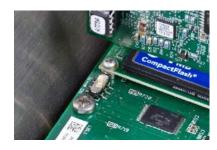
Figure 2-1: Metrology Switch, Location (left), shown in its OFF position (right)
