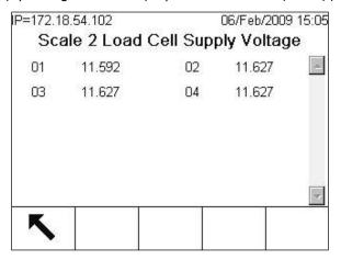
Figure 3-195: Scale Load Cell Supply Voltage Screen
