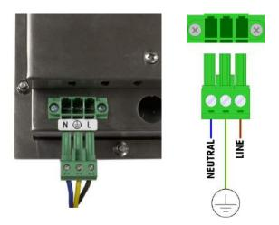
Figure A-31: Power Connector, Panel Mount Enclosure
