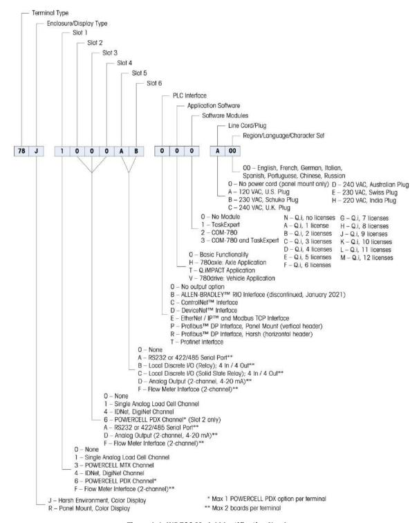
Figure 1-1: IND780 Model Identification Numbers
