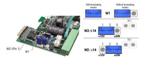
Figure A-47: POWERCELL MTX Card Jumper Locations and Settings
