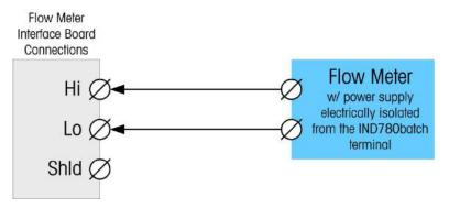
Figure A-79: Isolated Flow Meter Connections
