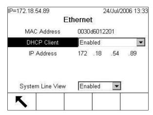
Figure 3-122: Ethernet Setup Screen, DHCP Client Enabled
