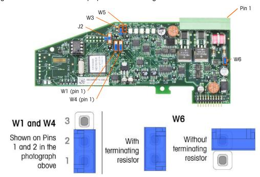
Figure A-50: POWERCELL PDX Board Jumper Locations and Settings
