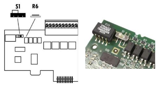
Figure A-81: Discrete I/O Board Mode Selector Switch Location
