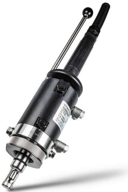
The retractable InTrac 77X housings accommodates 12 mm pH/ ORP, (dissolved) oxygen, and conductivity sensors. The housing has a flushing chamber in which the electrode can be rinsed, cleaned and recalibrated, without interference in the process. This housing features the patented Tri-Lock safety system for operational safety. The InTrac 77X is available with different process connections.
