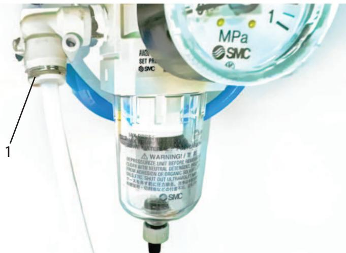
1. Air connection Rc 1/8, compatibility with 6mm tubing (quick connector)
