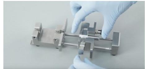
16 Take a new sleeve and align a slot of the sleeve with the guide pin of the SMART.
