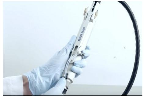
6 Hold the probe tip and turn the probe's outer tube to separate the shaft from the sleeve.
