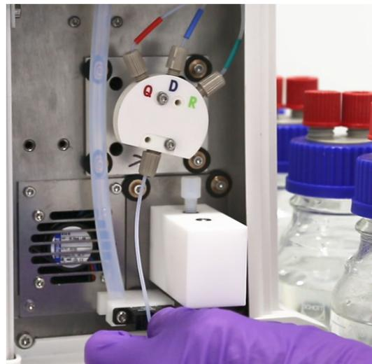
7 Connect the new tube from the pump to probe inlet (grey line). Ensure the color matches to the adapter lid.
