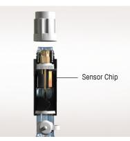
The instruments in the Titration Excellence line automatically recognize Plug & Play Sensors. All relevant data is saved in the Sensor Chip and automatically transferred to the titrator ensuring the correct sensor is being used at all times.
