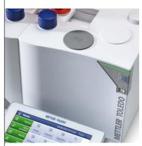
SmartChemical is an innovative product offered by METTLER TOLEDO that reinforces the concept of seamless workflows. All relevant chemical data such as name, batch number, or expiration date are stored on the chip placed below the chemicals label and transferred to the titrator with help of the integrated Smart reader. The automated data flow ensures its accuracy and completeness while saving operator time.
