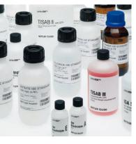
In all analytical procedures using an ISE, the correct amount of ISA (lonic Strength Adjustor) must be added to all samples and standards prior to measurement or calibration. This solution ensures that samples and standards have similar and constant ionic strength. Instructions for type and amount of ISA can be found in the manual of every ISE.
