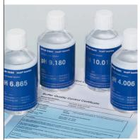
The NIST/DIN pH buffers are manufactured according to DIN/ISO 19266. They are specified to three decimal places, e.g. 9.180, offering the lowest possible uncertainty. A detailed test certificate is available for every bottle and guarantees the stated values and traceability.
