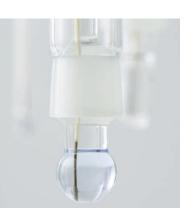
Thanks to the ARGENTHAL<sup>™</sup> reference system most METTLER TOLEDO pH sensors are filled with 3 mol/L KCI electrolyte solution. There is no longer a risk of contaminating your samples with silver ions. For measurements in non-aqueous samples or samples with low ionic strength a special bridge electrolyte is needed. Always make sure that your sensor is completely filled with clean electrolyte solution.
