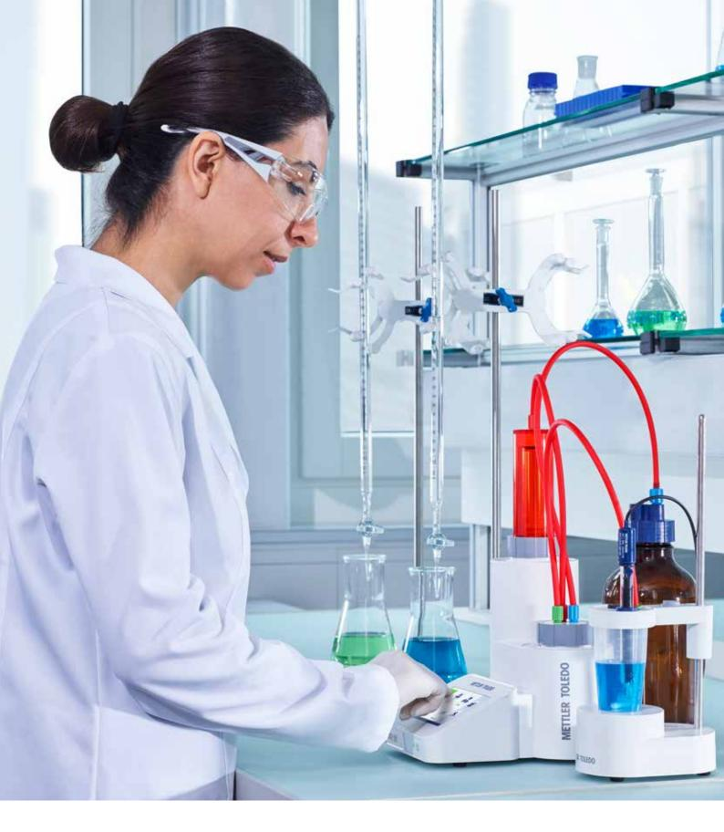
Reducing chemical and sample usage plays an important role in every laboratory. Titrations with an automated burette use smaller sample sizes and as a result use less titrant.
