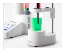
**Precise Measurements** Perform precise titrations with the automated burette and keep the focus on the color change of samples. An immersed dispensing tip further increases the precision, avoiding drop to drop variations.
