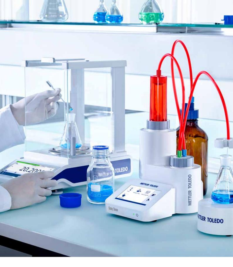
Minimize transcription errors by connecting the instrument to an MS, ML, or ME balance from METTLER TOLEDO and take advantage of automatic weight transfers.
