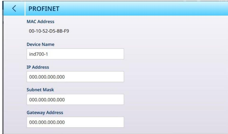
**Figure 3-9: PROFINET Setup Menu**
