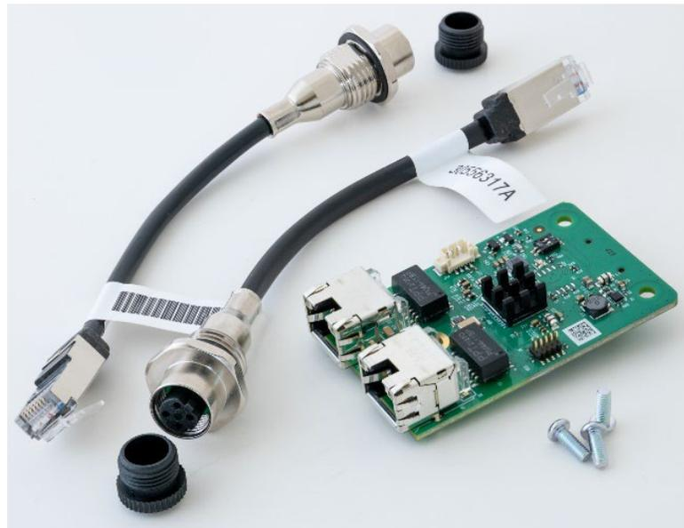
Figure 2-1: EtherNet/IP Interface Kit
