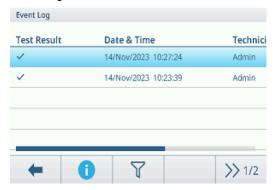
The Event Log records all planned actions from routine tests, including Calibration, Sensitivity, Eccentricity, and Repeatability, etc.
