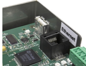
Figura 2-3: Puerto Ethernet IND780
