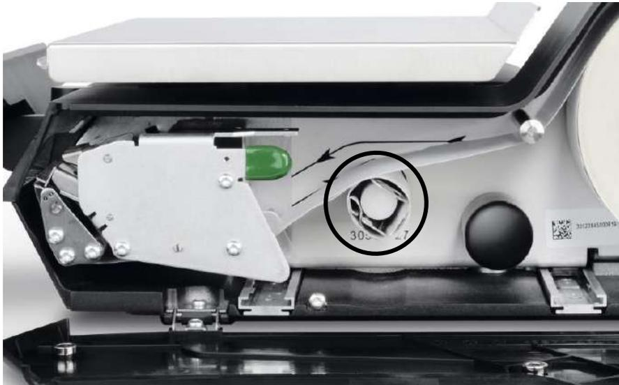
5. Lower and lock the print head and then push the printer back into its housing using the right side of the printer.
