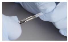
8 Expand the new tubing set slightly by using a tooth pick.
