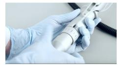
37 Place PTFE lines in the guide and connect the matching color-coded piece.
