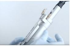
3 Unscrew and remove the nosepiece and collar.
