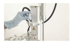
2 Fix the needle in place with the knurled screw.
