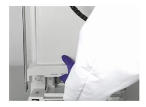
3 Remove tube from valve to pump.
