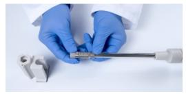
4 Place the probe tip with EasyFrit in the base of the installation tool. Make sure that the clamp nut remains outside of the tool while the filter main body sits well in its dedicated position.
