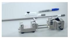
9 Slide the moving part of the SMART to reach the sample head intake.
