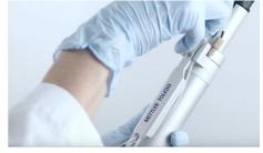
2 Slide the PTFE tubing out from the tube cover.
