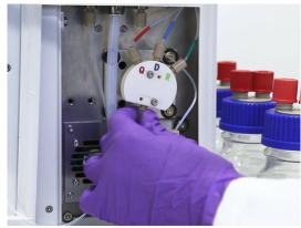
4 Remove tube from pump to probe inlet (grey line).
