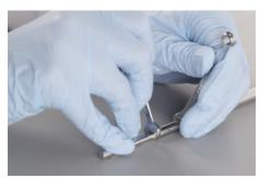
4 Manually unscrew the probe tube and pull back to reveal the tubing.
