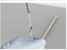
11 Orient the sampling head so that the pocket is facing up.
