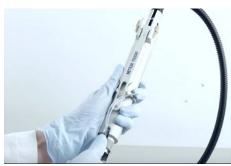
6 Hold the probe tip and turn the probe's outer tube to separate the shaft from the sleeve.
