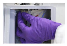
5 Remove tube from needle to probe outlet (black line).
