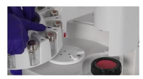
4 Rotate the rack lever clockwise to lock it in place.
