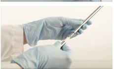
$25\ \mbox{Slide}$  the solvent lines through the Sleeve Mounting Clamp.
