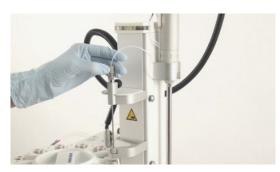
4 Mount the needle protection shield, taking care not to pinch the tubing.
