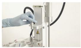
3 Connect the fitting nut to the needle and screw the fitting nut in until you hear a "click".
