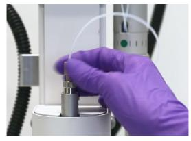
6 Connect the new tube from the valve to pump.
