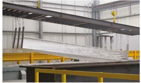
Hot-dip galvanizing coats the steel surface with a protective layer of zinc. By dipping the steel in a bath of molten zinc, the process covers the steel components completely, inside and out. Galvanized steel provides maintenance-free corrosion protection for the life of your scale.
