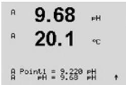
Enter the pH value of the sample then press the [ENTER] key to start the calculation of the calibration results.
