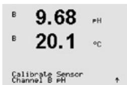
Enter pH calibration mode as described in section 7.1 "Enter Calibration Mode".
