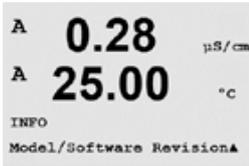
Selecting Model/Software Revision will display the part number, model and the serial number of the transmitter.
