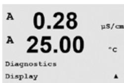
All pixels of the display will be lit for 15 seconds to allow troubleshooting of the display. After 15 seconds the transmitter will return to the normal measuring mode or press [ENTER] to exit sooner.
