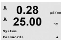
This menu allows for the configuration of operator and administrator passwords, as well as setting up a list of allowed menus for the operator. The administrator has rights to access all menus. All default passwords for new transmitters are “00000”.
