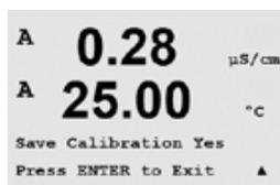
Press [ENTER] to bring up a confirmation screen. Select Yes to save the calibration values and the successful calibration is confirmed on the display.
