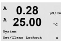
This menu enables/disables the lockout functionality of the transmitter. The user will be asked for a password before being allowed into any menus if the lockout functionality is enabled.
