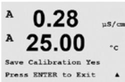
Pressing the [ENTER] key after entering Point 2 will bring up a confirmation screen. Select Yes to save the calibration values and the successful calibration is confirmed on the display. The transmitter will return to the measurement mode in approximately 5 seconds.
