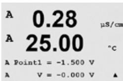
Enter the value for Point 1 in, volts, connected to the input. The second display line will show the measured voltage. Press[ENTER] to begin the calibration process.
