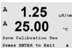
Select Yes to save the new calibration values and the successful calibration is confirmed on the display.
