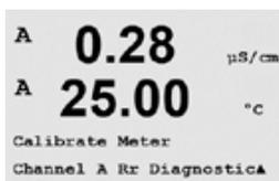
Rr diagnostic is performed as a two point calibration. Navigate to the Calibrate Meter screen and select Channel A and Rr Diagnostic.
