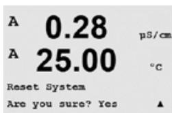
Pressing the [ENTER] key after the selection will bring up a confirmation screen. Selecting No will return the user to the measurement mode with no changes, while selecting Yes will reset the meter.
