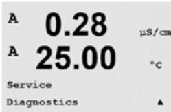
This menu is a valuable tool for troubleshooting and provides diagnostic functionality for the following items: Model/Software Revision, Digital Input, Keypad, Memory, Set OC, Read OC, Set Analog Outputs, Read Analog Outputs.
