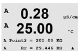
Enter the value for Point 2 of the calibration according to the resistor connected across the pH reference measuring input.
