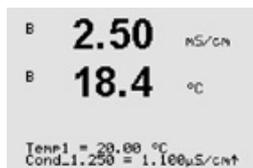
Enter the value of the 1st temperature (**Temp1**) and the value for the conductivity which belongs to the first concentration at this temperature.
