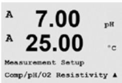
Depending on the connected sensor, the menu can be selected by using the A or ▼ key. Press [ENTER]
