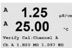
The measured signal of the primary and the secondary measurement in electrical units are shown. The meter calibration factors are used when calculating these values.
