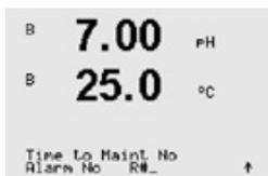
**Time to Maintenance:** This timer estimates when the next cleaning cycle should be performed to keep the best possible measurement performance. The timer is influenced by significant changes on the DLI parameters.
