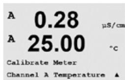
Temperature is performed as a three point calibration. The table above shows the resistance values of these three points.
