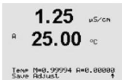
Select ADJUST or ABORT to finish calibration. See "7.1.2 Finish Calibration".
