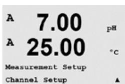
Press the [ENTER] key to select the "Channel Setup" menu.
