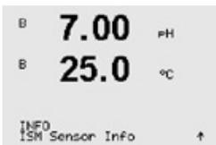
After plugging in an ISM sensor it is possible by using the key A or ▼ to navigate to the Menu "ISM Sensor Info".
