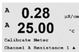
The M400 transmitter is factory calibrated within specifications. It is not necessary to perform meter re-calibration unless extreme conditions cause an out of spec operation shown by Calibration Verification. Periodic verification/re-calibration may also be necessary to meet Q.A. requirements. Meter calibration can be selected as current (used for most dissolved oxygen, Voltage, Rg Diagnostic, Rr Diagnostic (used for pH), and temperature (used for all measurements).
