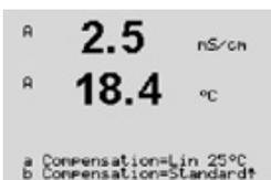
Lin 25 °C compensation adjusts the reading by a factor expressed as a "% per °C" (deviation from 25 °C). Use only if the solution has a well-characterized linear temperature coefficient.
