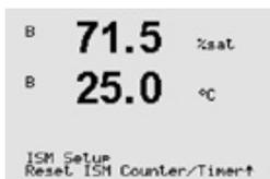
Navigate to the menu "Reset ISM Counter/Timer" by using the ▲ and ▼ keys and press [ENTER].
