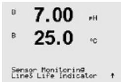
The sensor monitoring allows you to display the sensor monitoring details on line 3 and 4 in the display. The following options are possible:
