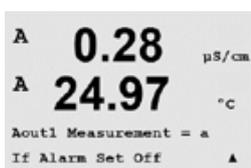
When an alarm value is selected (see chapter 8.5.1 "Alarm"; PATH: Menu/Configure/Alarm/Clean/Setup Alarm), the analog output will go to this value if any of these alarm conditions occurs.
