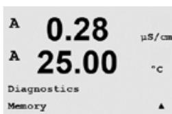
If Memory is selected then the transmitter will perform a RAM and ROM memory test. Test patterns will be written to and read from all RAM memory locations. The ROM checksum will be recalculated and compared to the value stored in the ROM.
