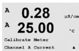
Current calibration is performed as a two point calibration.
