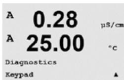
For keypad diagnostics, the display will indicate which key is pressed. Pressing [ENTER] will return the transmitter to the normal measuring mode.
