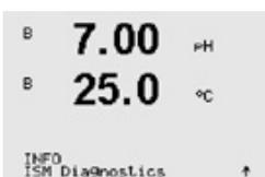
After plugging in an ISM sensor it is possible by using the key A or ▼ to navigate to the Menu "ISM Diagnostics".
