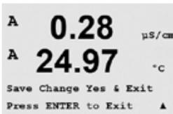
Pressing the [ENTER] key again will bring up the Save Changes dialog. Selecting No will discard the entered values and return to the measurement display screen, while selecting Yes will save changes made.
