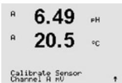
Enter mV calibration mode as described in section 7.1 "Enter Calibration Mode".
