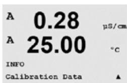
Selecting Calibration Data displays the calibration constants for each sensor.
