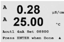
As the five digit number is increased the output current increases and as the number is decreased the output current decreases. Thus coarse changes in the output current can be made by changing the thousands or hundreds digits and fine changes can be made by changing the tens or ones digits.
