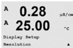
This menu allows the setting of the resolution of each displayed value.
