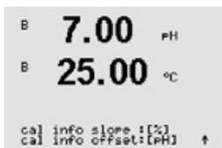
The units for the slope and the zero point that will be shown on the display can be chosen. The default setting for the unit of the slope is [%] and can be changed to [pH/mV]. For the zero point the default setting of the unit is [pH] and can be changed to [mV]. Use the ► key to move to the input field and select the unit by using the ▲ or ▼ key.
