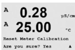
Pressing the [ENTER] key after the selection will bring up a confirmation screen. Selecting No will return the user to the measurement mode with no changes, while selecting Yes will reset the meter calibration factors.
