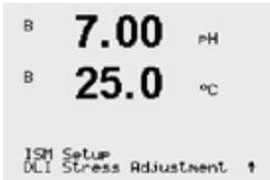
Navigate to the menu "DLI Stress Adjustment" by using the ▲ and ▼ keys and press [ENTER].
