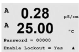
The lockout-menu is protected: Enter the administrator or operator password and select YES to enable or NO to disable the lockout functionality. Pressing the [ENTER] key after the selection will bring up the Save Changes dialog. Selecting No will discard the entered value, while selecting Yes will make the entered value the current one.
