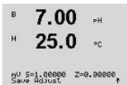
The display shows the slope calibration factor "S" and the offset calibration factor "Z".
