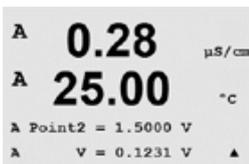
Enter the value for Point 2, in volts, of the source connected to the input. The second display line shows the measured voltage.
