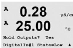
The **"DigitalIn"** function applies all the time. As soon as a signal is active on the digital input the transmitter goes to hold mode and the values on the analog output, the output OC will be at hold state.
