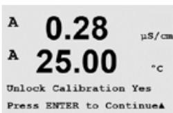
Selecting Yes means that meter and analog output calibration menus will be selectable under the CAL Menu. Selecting No means that only the sensor calibration is available under the CAL Menu. Press [ENTER] after the selection to display a confirmation screen.
