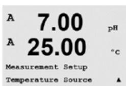
Enter Measurement as described in chapter 8.2 "Measurement". Select Temperature Source by using the ▲ or ▼ key and press [ENTER].
