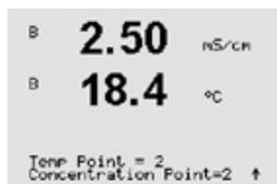
Enter the amount of desired temperature points "Temp Point" and "Concentration Points".
