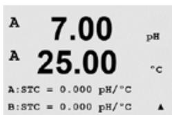
**STC** is the solution temperature coefficient in units of pH/°C referenced to 25 °C (Default = 0.000 for most applications). For pure waters, a setting of 0.016 pH/°C should be used. For low conductivity power plant samples near 9 pH, a setting of 0.033 pH/°C should be used. These positive coefficients compensate for the negative temperature influence on the pH of these samples. Press [ENTER].
