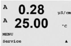
While in measurement mode press the ◀ key. Press the ▲ or ▼ key to navigate to the “Service” menu and press [ENTER]. The available system configuration options are detailed below.
