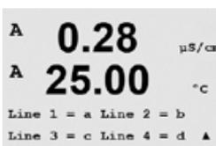
Select the "Error Display" mode. If this is set to "On" when an alarm or warning has occurred, the message "Failure – Press ENTER" will be displayed on Line 4 when an alarm occurs in the normal measurement mode.
