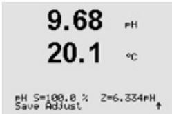
After the calibration the slope calibration factor "S" and the offset calibration factor "Z" are displayed.
