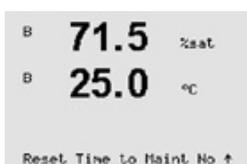
If an pH sensor is connected, the menu for resetting the Time To Maintenance is displayed. Time To Maintenance needs to be reset after the following operations.
