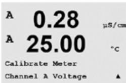
Voltage calibration is performed as a two point calibration.
