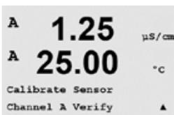
Enter Calibration mode as described in section 7.1 "Enter Calibration Mode" and select Verify.
