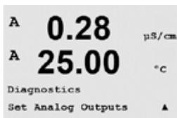
This menu enables the user to set all analog outputs to any mA value within the 0–22 mA range. Press [ENTER] to exit from this display.
