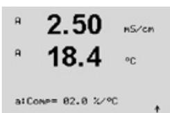
If compensation mode "Lin 25 °C" or "Lin 20 °C" has been chosen, the factor for the adjustment of the reading can be modified after pressing [ENTER] (If working at measurement line 1 or 2 press [ENTER] twice).
