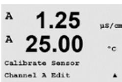
Enter Calibration mode as described in section 7.1 "Enter Calibration Mode" and select Edit, Edit pH, Edit mV.
