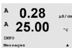
Pressing the ▼ key will display the Info menu with the options Messages, Calibration Data and Model/Software Revision.
