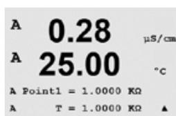
The first text line will ask for the Point 1 temperature resistance value (this will correspond to temperature 1 value shown on the calibration module accessory). The second text line will show the measured resistance value. When the value stabilizes, press [ENTER] to perform calibration.
