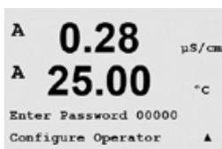
See 9.3 on how to enter the passwords Menu. Select Configure Operator to configure the access list for the operator. It is possible to assign/deny rights to the following menus: Cal Key, Quick Setup, Configuration, System, PID Setup and Service.
