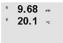
After determining the pH value of the sample, press the [CAL] key again to proceed with the calibration.
