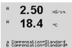
Standard compensation includes compensation for non-linear high purity effects as well as conventional neutral salt impurities and conforms to ASTM standards D1125 and D5391.
