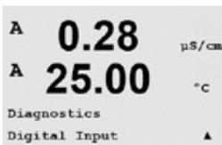
The digital input menu shows the state of the digital inputs. Press [ENTER] to exit from this display.
