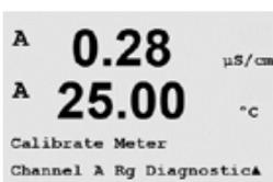
Rg diagnostic is performed as a two point calibration. Navigate to the Calibrate Meter screen and select Channel A and Rg Diagnostic.
