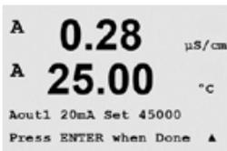
Connect an accurate milliamp meter to the analog output terminals and then adjust the five digit number in the display until the milliamp meter reads 4.00 mA and repeat for 20.00 mA.
