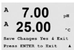
Selecting No will discard the entered values and return to the measurement display screen, while selecting Yes will save changes made.
