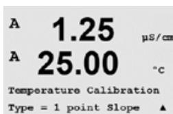
Select one-point calibration. Slope or Offset can be selected with the one-point calibration. Select Slope to recalculate the Slope factor "M" (Multiplier) or Offset to recalculate the offset calibration factor "A" (Adder).
