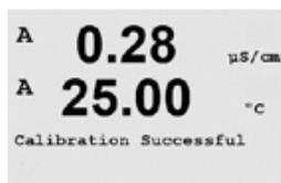
The transmitter will return to the measurement mode in approximately 5 seconds.
