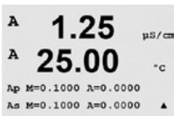
All calibration constants for the selected sensor channel are displayed. Primary measurement constants (p) are displayed on Line 3. Secondary measurement (temperature) constants (s) for the sensor are displayed on Line 4.
