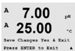
After the procedure of the channel setup described in the previous chapter pressing the [ENTER] key again will bring up the Save Changes dialog. Selecting No will discard the entered values and return to the measurement display screen, while selecting Yes will save changes made.
