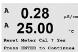
This menu allows the reset of the meter's calibration factors to the last factory calibration values.
