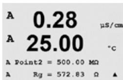
Enter the value for Point 2 of the calibration according to the resistor connected across the pH glass electrode measuring input.
