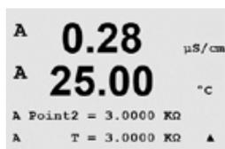
The transmitter screen will then prompt the user to enter the value for Point 2, and T2 will display the measured resistance value. When this value stabilizes, press [ENTER] to calibrate this range.
