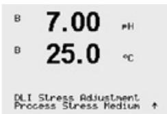
Adjust the Process Stress parameter based on the particular application and/or requirements
