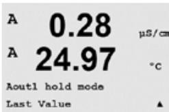
The value for the Hold mode can be configured to hold the last value or can be set to a fixed value.
