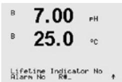
**Lifetime indicator:** The dynamic lifetime indication allows an estimation, when the pH electrode is at the end of his lifetime, based on the actual stress he is exposed to. The sensor permanently takes the averaged stress of the past days into consideration and is able to increase/decrease the lifetime accordingly.
