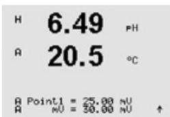
The user can now enter Point 1. The offset calibration factor is calculated by using the value of Point1 instead of the measured value (line 4, mV = ....) and displayed on the next screen.
