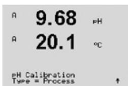
Select Process calibration. With pH sensors a process calibration is always performed as an offset calibration.
