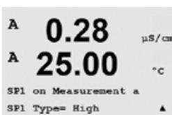
Up to 6 setpoints can be configured on any of the measurements (a thru d). The possible Setpoint types are Off, High, Low, Outside (<->) and Between (>-<).
