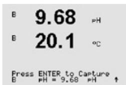
Take a sample and press the [ENTER] key again to store the current measuring Value. To show the ongoing calibration process, "A" or "B" (depending on the channel) will blink in the display.
