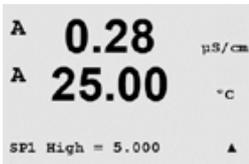
Depending on the defined setpoint type, this screen provides the option to adjust the values for the setpoint(s).
