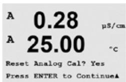
This menu allows reset of the analog output calibration factors to the last factory calibration values.
