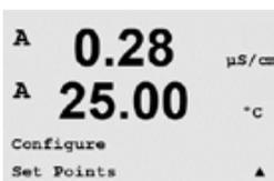
Enter Configuration mode as described in Section 8.1. "Enter Configuration Mode" and navigate to the menu "Set Points" by using the ▲ or ▼ key.
