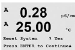
This menu allows the reset of the meter to the factory default settings (setpoints off, analog outputs off, etc.). The meter calibration and the analog output calibration are not affected.
