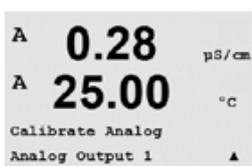
Select the Analog Output you wish to calibrate. Each analog output can be calibrated at 4 and 20 mA.
