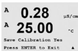
Pressing the [ENTER] key after entering Point 2 will bring up a confirmation screen. Select Yes to save the calibration values and the successful calibration is confirmed on the display. The transmitter will return to the measurement mode in approximately 5 seconds.
