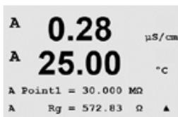
Enter the value for Point 1 of the calibration according to the resistor connected across the pH glass electrode measuring input. Press [ENTER] to begin the calibration process.
