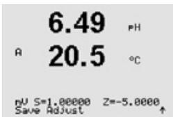
"Z" is the newly calculated offset calibration factor. The slope calibration factor "S" is always 1 and does not enter the calculation.
