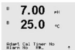
Activation of the **Adaptive Calibration Timer:** This timer estimates when the next calibration should be performed to keep the best possible measurement performance. The timer is influenced by significant changes on the DLI parameters.
