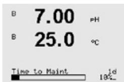
**Time to Maintenance:** This timer shows when the next cleaning cycle should be performed to keep the best possible measurement performance. The Time to Maintenance is indicated in days (d) and percentage (%). For a description of the Time to Maintenance, please see section 8.6 "ISM Setup". For oxygen sensors, the Time to Maintenance indicates a maintenance cycle for the membrane and electrolyte.
