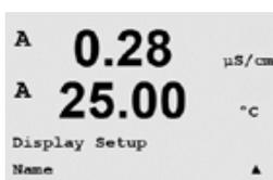
This menu allows for the configuration of an alpha-numeric name which is displayed in the first 9 characters on lines 3 and 4 of the display. The default is nothing (blank).
