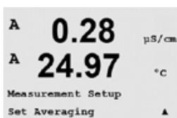
The averaging method (noise filter) for each measurement line can now be selected. The options are Special (Default), None, Low, Medium and High:
