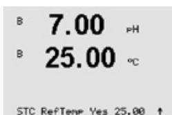
**STC RefTemp** sets the temperature to which solution temperature compensation is referenced. The displayed value and the output signal is referenced to STC RefTemp. Selecting "No" means solution temperature compensation is not used. The most common reference temperature is 25 °C. Press [ENTER].
