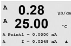
Enter the value for Point 1, in milliamps, of the current source connected to the input. The second display line will show the measured current. Press [ENTER] to begin the calibration process.
