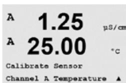
Enter Sensor calibration mode as described in section 7.1 "Enter Calibration Mode" and select Temperature.
