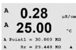
Enter the value for Point 1 of the calibration according to the resistor connected across the pH reference measuring input. Press [ENTER] to begin the calibration process.
