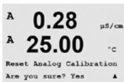
Pressing the [ENTER] key after the selection will bring up a confirmation screen. Selecting No will return the user to the measurement mode with no changes, while selecting Yes will reset the analog output calibration.
