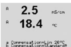
Lin 20 °C compensation adjusts the reading by a factor expressed as a "% per °C" (deviation from 20 °C). Use only if the solution has a well-characterized linear temperature coefficient.
