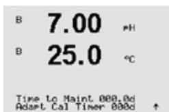
The initial value for Time to Maintenance as well as the Adaptive Calibration Timer can be modified according to the application experience and loaded down to the sensor.
